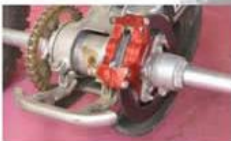
Disco + pinza + pastilla disc + caliper + bracket
