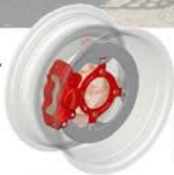
Pinza y disco de la rueda delantera (llanta 10") disc and caliper in the front wheel (10" wheel)
